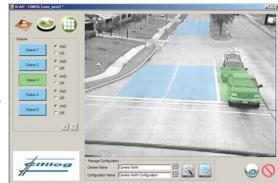
The XCam-p can be installed up to a distance of 300m from the XCom, which is typically installed in the traffic controller cabinet. A wireless module enables a wireless connection of several XCam-p video sensors.
